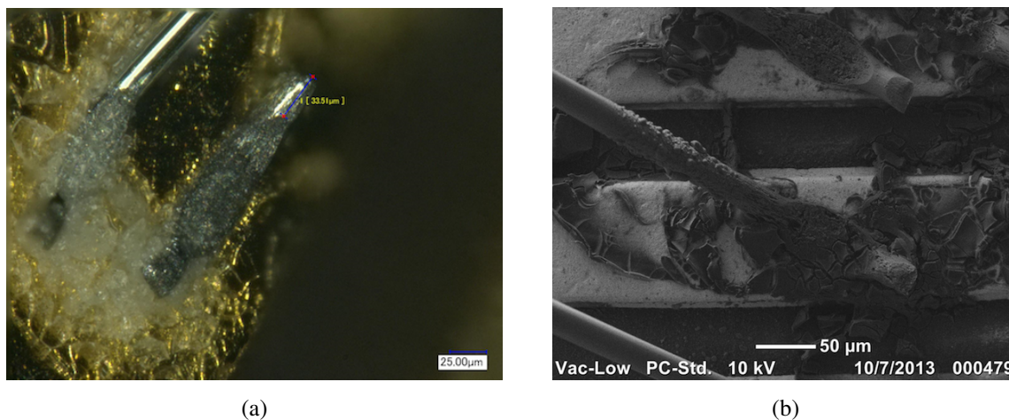
Figure 46. (a) White residue of corrosion on staves as observed under a microscope. (b) A Scanning Electron Microscopy (SEM) image of corroded wires and the corrosion residue at the foot of the bond.
