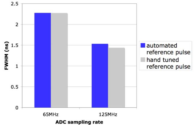
Fig. 9. Result of coincidental timing for the hand-tuned reference pulse derived from 25GHz oscilloscope data (grey) and a reference pulse from our automated algorithm (blue).
