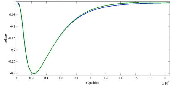
Fig. 8. Matlab plot of two reference pulses. The green pulse is derived from our algorithm while the blue pulse is derived from 25GHz oscilloscope data.
