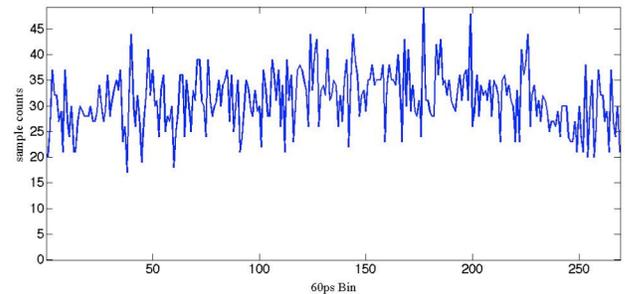
Fig. 6. Histogram of the distribution of pulse samples over one ADC interval (0-255) for the higher resolution pulse.
