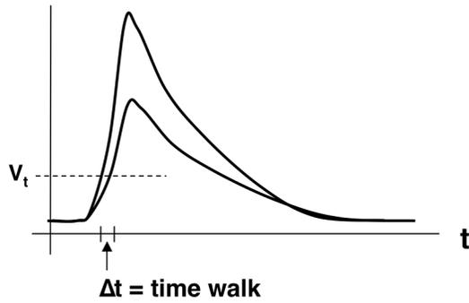
Fig. 1. Illustration of the timing jitter introduced by time walk when two pulsed have varying amplitudes.
