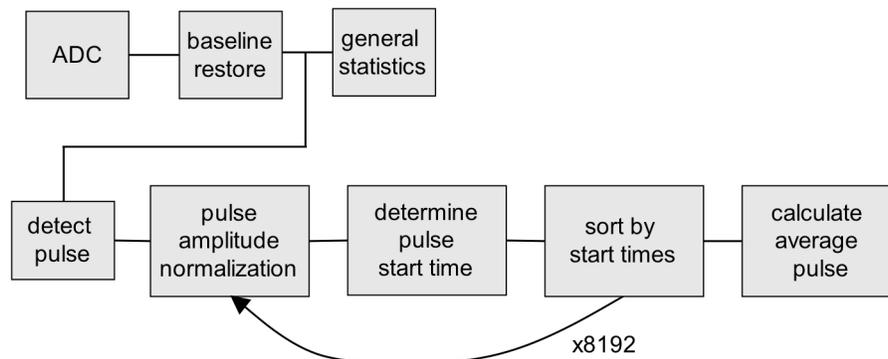
Fig. 3. Block diagram of the overall reference pulse discovery algorithm.
