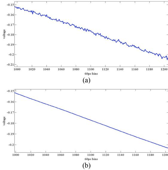
Fig. 7. Matlab plot of 12ns of the leading edge of the derived reference pulse (a) before smoothing and (b) after smoothing.
