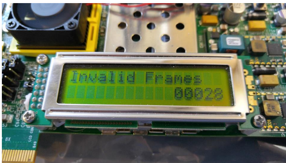
Figure 3.17: Invalid frames displayed on LCD screen. Image depicts invalid frames being sent deliberately to test proper functionality of LCD.
