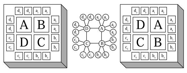
**Figure 4.** An example of a local minima in placement. The circuit at center, placed as shown at left, is in a local minima. No swap of logic or I/O functions will reduce the total wirelength. However, the placement at right is significantly better.
