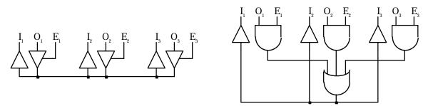
**Figure 24.** Tristate buses (left) in circuits mapped to multi-FPGA systems can be converted to a logic structure with only single-source nets (right) [Butts91].
