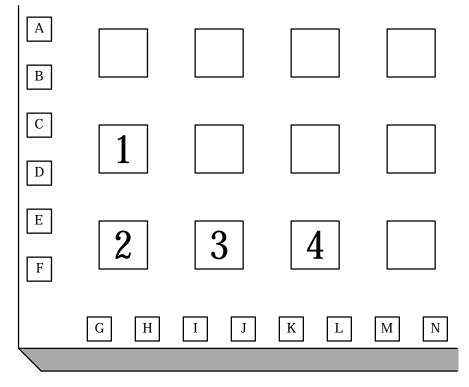
**Figure 3.** Placement of the circuit from Figure 2. The numbers are the number of the LUT (from the technology mapping) assigned to each logic block, while the letters are the assignment of input signals to I/O blocks.
