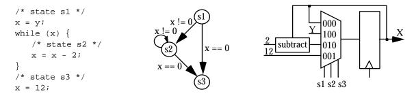
**Figure 25.** Example of variables and complex control flow. The code segment (left) is converted into a control state machine (center) and logic for controlling the variable's register (right). Although the states are shown in the code, these are automatically inferred from the control flow.
