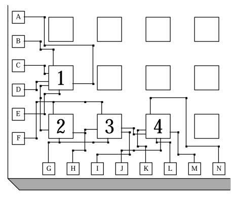
**Figure 5.** Routing of the placement from Figure 3. The small black squares are the configuration points used for this mapping.
