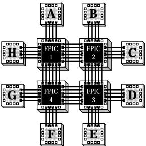
Figure 22. Multi-FPGA topologies with simple pin assignments.
