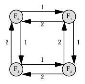
Figure 13. FPGA channel graph showing the initial values of the available channel capacities.
