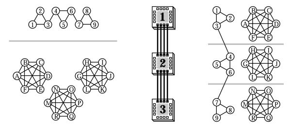
**Figure 7.** An example of the suboptimality of recursive bipartitioning. We are partitioning to the multi-FPGA system at middle, and the best first cut is shown at left (gray line). The next partitioning would have to cut nine signals. We can instead partition as shown at right, cutting a total of two signals.
