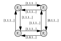
**Figure 20.** FPGA channel graph showing the values of the available channel capacities after wire *a* has been scheduled.
