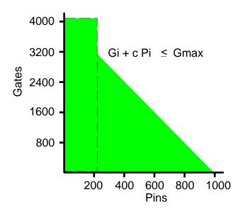
Figure 10. Constraints used by a VirtualWires partitioner.
