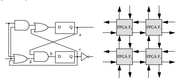
Figure 17. Input circuit (left) and FPGA topology (right).
