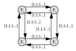
**Figure 18** FPGA channel graph showing the initial values of the available channel capacities as a function of the virtual cycle. Initially,  $C^{a}(t)$  for each channel is 1 for all values of t.
