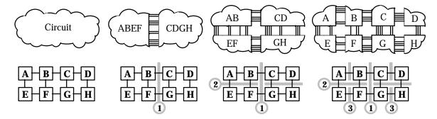
**Figure 8.** Example of iterative bipartitioning. The circuit (top left) is partitioned onto the multi-FPGA topology (bottom left) in a series of steps. Each partitioning corresponds to the most critical bottleneck remaining in the multi-FPGA system, and after each partitioning the placement of the logic is restricted to a subset of the topology (labeling on circuit partitions).
