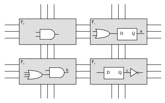
Figure 14. A partition and placement of the input circuit.
