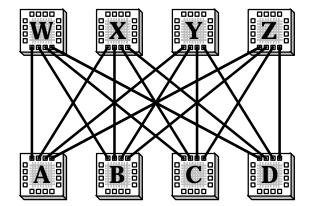
**Figure 11.** Crossbar routing topology. The chips at top are used purely for routing, while the FPGAs at bottom handle all the logic in the system.
