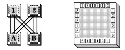
**Figure 23.** Topology for integrated global routing and pin assignment (left), with the FPGAs at bottom used for logic, and the FPGAs at top for routing only. The detailed pin connections of the logic-bearing FPGAs are given at right. The numbers in the pin positions indicate to which routing-only chip that pin is connected.
