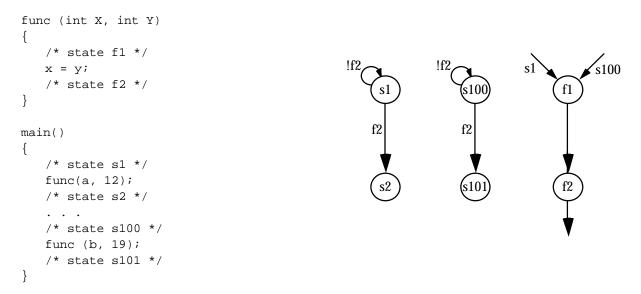
**Figure 26.** A code segment with a function call (left) is converted into a separate FSM for each procedure (right), with appropriate communication between components.
