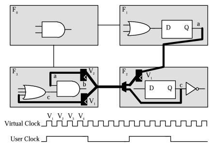
**Figure 21.** Virtual routing of wires a and c. On virtual cycle V1, the signal on wire a is routed from F1 to intermediate hop F2, and the signal on wire c is routed from F2 to F3. The figure also shows the multiplexing and hop logic introduced by VirtualWires to implement the routing and scheduling.
