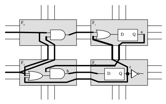
Figure 16. A routing of the input circuit on the target topology.
