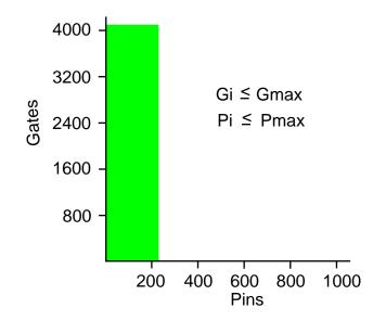
Figure 9. Constraints used by a traditional partitioner.
