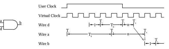
Figure 19. The relationship between the various scheduling times for signals a, d, and b. Wire b depends combinationally upon a and d, and a is produced as the output of a flip flop.
