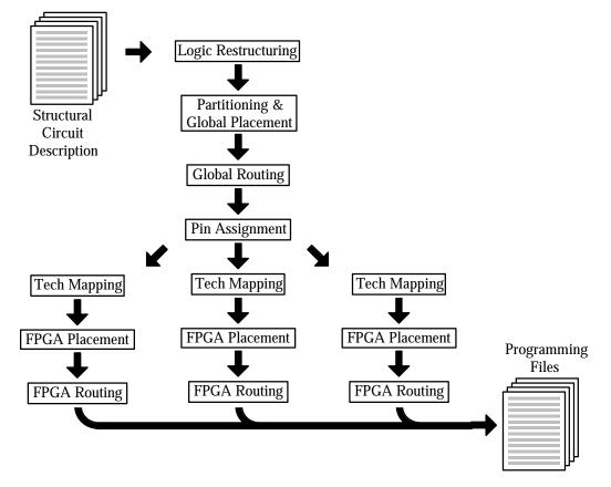
Figure 1. Multi-FPGA system mapping software flow.
