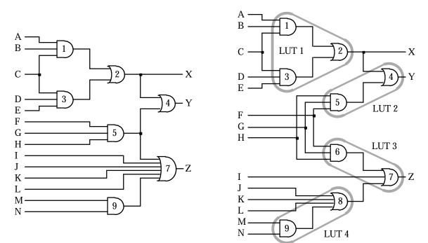
**Figure 2.** Example of 5-input LUT technology mapping. The input circuit (left) is restructured and grouped together into 5-input functions (right). The gray loops at right indicate individual LUTs. The numbers on the gates are for identification.
