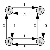
Figure 15. Channel graph showing available channel capacities after routing the net a.
