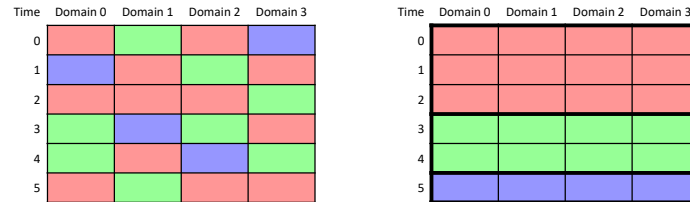
Figure 10. Example modulo schedule after flattening and IMS scheduling (left) and modulo schedule organized by mode (right).
