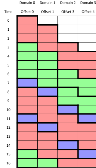
Figure 13. Offset Pipelining execution trace of Figure 12 schedule.
