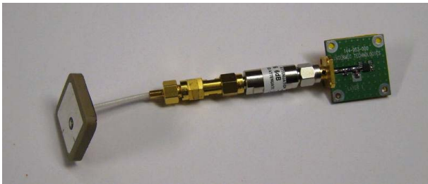
Figure 11. Small ceramic patch antenna connected to RFID IC assembly.
