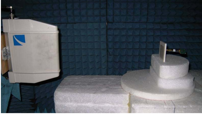
Figure 10. Gain measurement based on passive RFID characterization setup.
