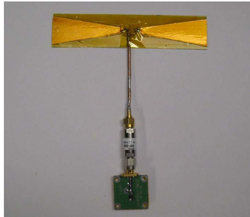
Figure 6. Reference dipole antenna connected to 50 Ohm RFID IC assembly.
