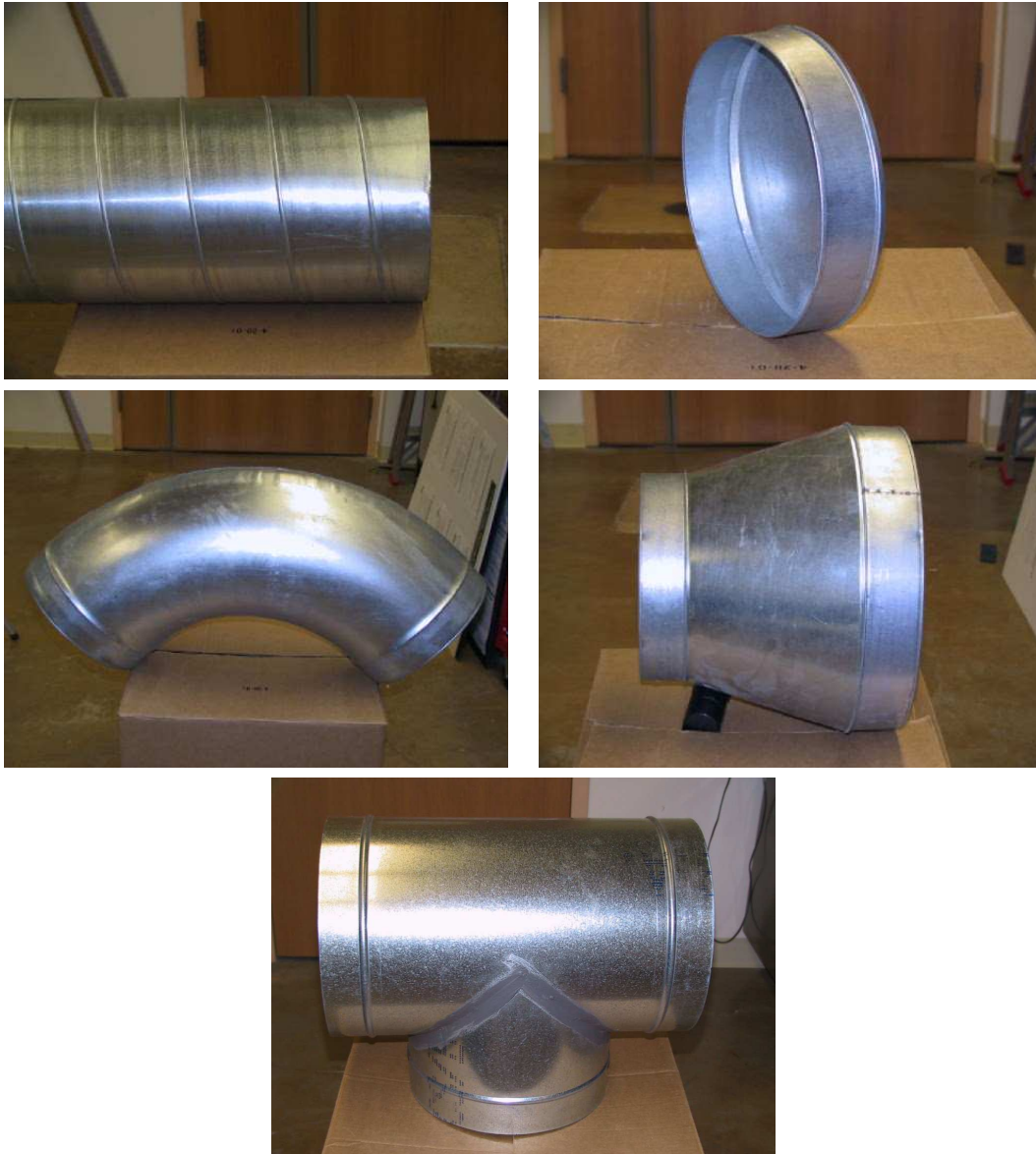
Figure 6.6: Straight section, metal end cap, bend, taper, and T-junction used in experiments.
