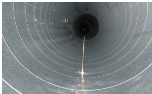
Fig. 6. Monopole antenna in the duct used for channel testing.
