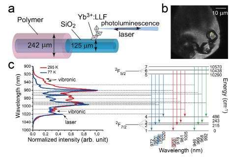
**Figure 2.** a) Schematic of  $10\%Yb^{3+}$ :LLF microcrystals on a SiO<sub>2</sub> optical fiber in vacuum; b) Optical micrograph of  $10\%Yb^{3+}$ :LLF microcrystals on a SiO<sub>2</sub> optical fiber; c) Assignment of the crystal-field transitions of Yb<sup>3+</sup> in LLF following excitation with a pulsed laser at  $\lambda = 1020$  nm.
