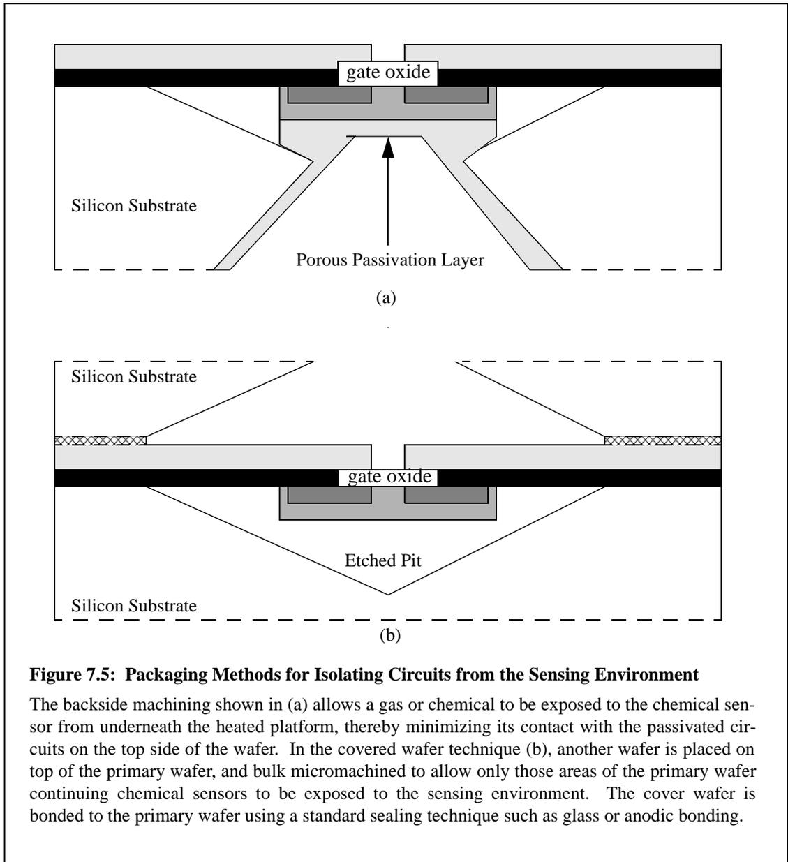
**Figure 7.5: Packaging Methods for Isolating Circuits from the Sensing Environment**
