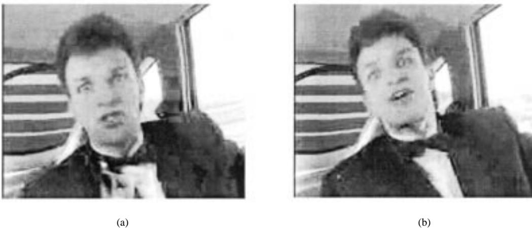
Fig. 10. Subjective evaluation for 32 kb/s "Carphone" sequence. Reduce number of packet errors from interleaving with PSNR improvement of 4.5 dB for frame #21. (a) TMN-8 and (b) proposed conditional retransmission and interleaving scheme.
