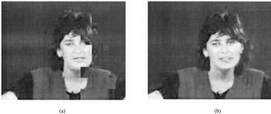
Fig. 9. Subjective evaluation for 32 kbits/s "Miss America" sequence. Reduce number of packet errors from interleaving with PSNR improvement of 7.5 dB for: (a) frame #31. (a) TMN-8 and (b) proposed conditional retransmission and interleaving scheme.
