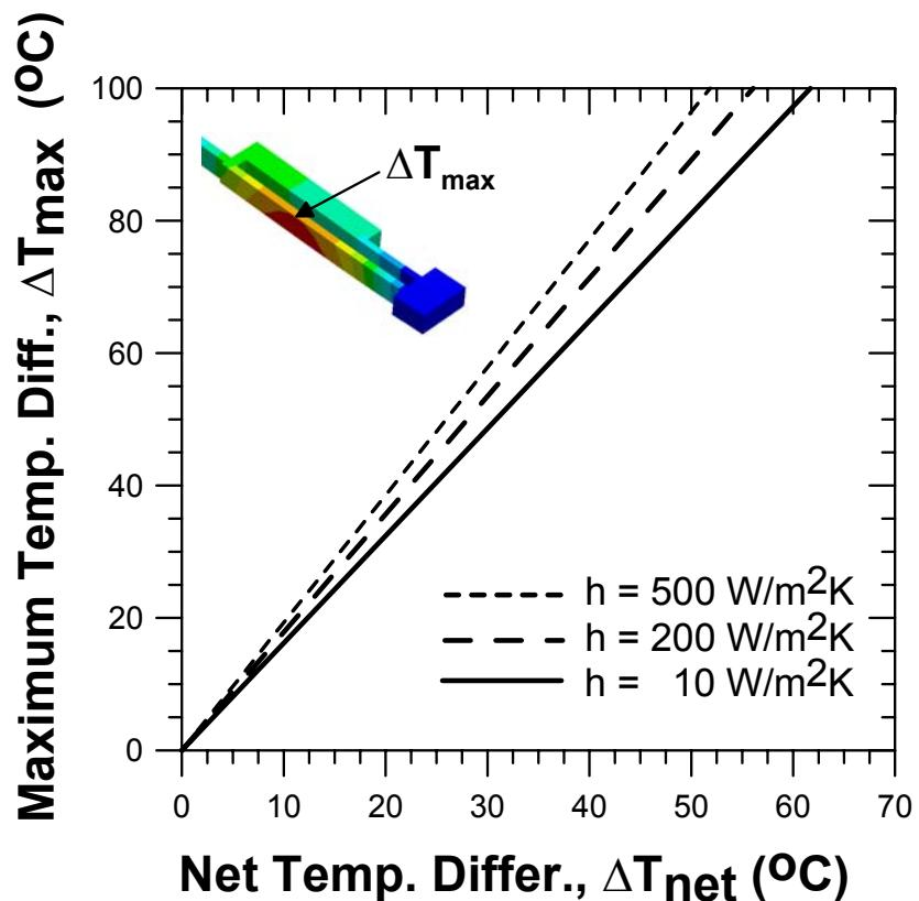
**Net Temperature Difference:**  $\Delta T_{net} = \frac{1}{L_1 + L_2 + L_3} \left[ \int_0^{L_h} T_{hot} dx + \int_0^{L_c} T_{cold} dx + \int_0^{L_f} T_{flexure} dx \right]$
