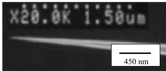
Figure 6. An ultrasharp tungsten probe end-effector used for electrical probing and physical manipulation of nano-scale objects.
