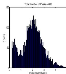
Figure 4. Distribution of voltage peaks obtained with a suspension of NT8e cells (1 $\times$ 10<sup>5</sup> cells/ml). Compared with the standard particles, using particle volume scaling, the mean cell diameter can be estimated from to be  $\sim$ 17 $\mu$ m.
