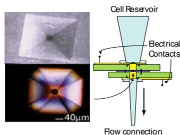
Figure 2. SEM and optical micrographs of the fabricated *sense-porate aperture* – a thermally oxidized anisotropically etched through hole in silicon. This is mounted between PCBs with gold-plated electrodes and plastic flow connectors.
