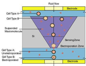
Figure 1. Principle of in-flow selective electroporation in a microfabricated *sense-porate aperture*. Cells moving through the tapered aperture are sensed and identified by their impedance and then electroporated in a selectively triggered controlled electric field zone.
