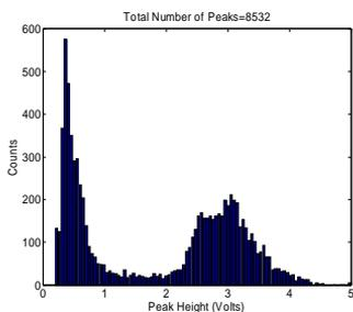
Figure 3. Distribution of voltage peaks obtained with a mixture of polystyrene particles with nominal diameters of 10 $\mu$ m and 20 $\mu$ m. The mean peak heights roughly scale according to particle volume ( $\propto r^3$ ) as expected theoretically.
