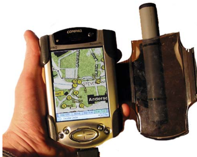
Fig. 4. Integrated PDA and RFID hand-held device for the UW Electronic Tree Tour. The screen shows part of the campus map with trees identified with numbered circles. The RFID wand extends to the right of the PDA. The user carries the reader and batteries in a hip pack.
