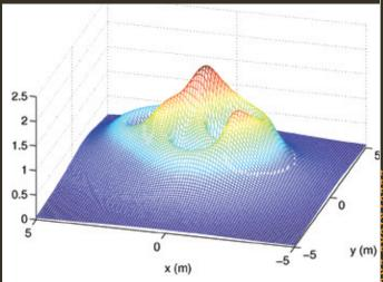
The surface represents the aggregation of RSS measurements from three beacons to indicate the device's probable location.
