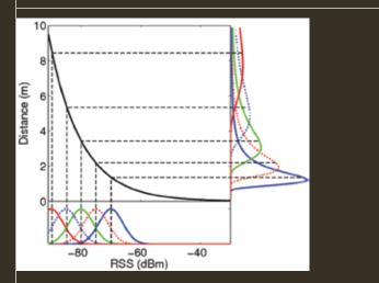
The mapping from RSS measurements to distance estimates can be used to map the Gaussian distribution of RSS measurement error to a distribution of the beacon distance. Note that RSS measurements from distant beacons have high estimation variance illustrated by the wide distribution whereas RSS measurements from nearby beacons have low estimation variance as illustrated by the narrow distribution.
