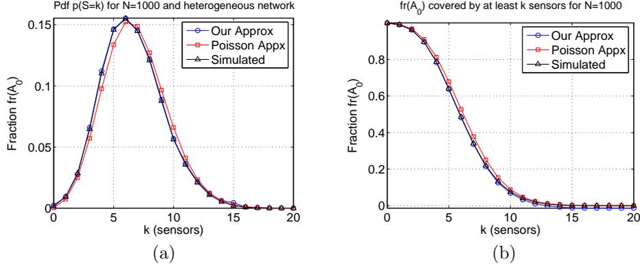
Fig. 12. Heterogeneous sensor network, with  $FoI$  being a disk of radius  $R = 100m$ . An equal number of two types of sensors are deployed; Type  $A$  has a sensing area of a disk shape with radius  $r_A = 10m$ , while type  $B$  has a sensing area of a disk shape with  $r_B = 15m$ . (a) The pdf of the fraction  $fr(\mathcal{A}_0)$  covered by exactly  $k$  sensors when  $N = 500$  sensors. (b) The fraction  $fr(\mathcal{A}_0)$  covered by at least  $k$  sensors when  $N = 500$  sensors.
