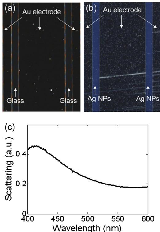
FIG. 2. (Color online) Plasmonic Ag NP deposition by self-assembly process. Dark field images of an electrode-patterned substrate (a) before, and (b) after Ag NP deposition. (c) Dark field scattering spectrum of Ag NPs on glass substrate. A resonance is shown at 415 nm.
