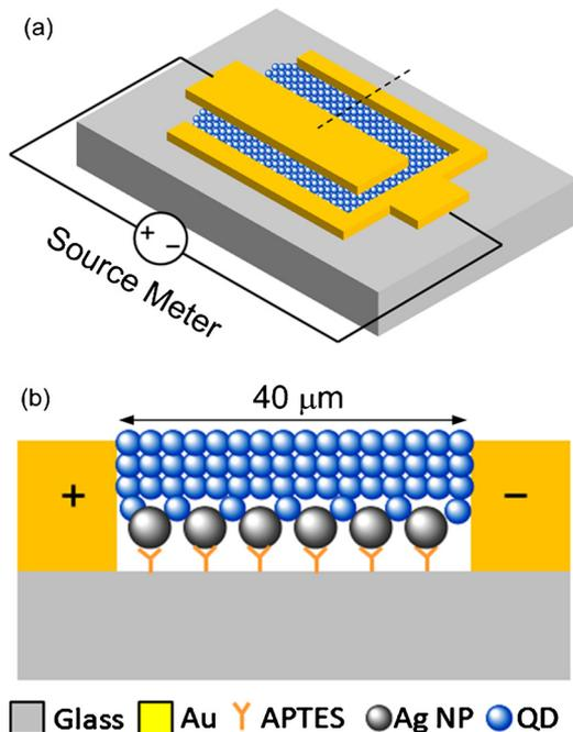
FIG. 1. (Color online) Schematic drawings of a plasmonic QD photodetector. (a) 3D top view schematics, and (b) cross-section view along the dash line in Fig. 1(a).
