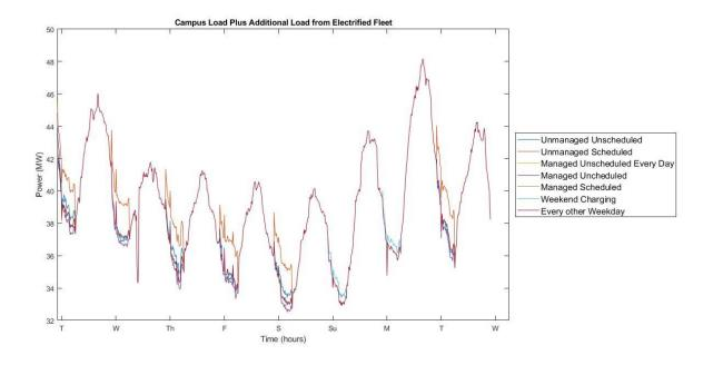
Figure 5.5. Total Hourly Campus Load Including Electrified Fleet Load
