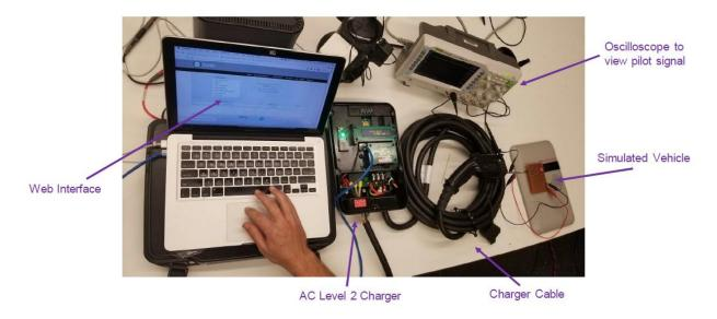
Figure 2.4. Capstone Test Setup
