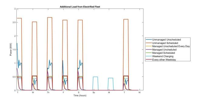
Figure 5.4. Electrified Fleet Hourly Load
