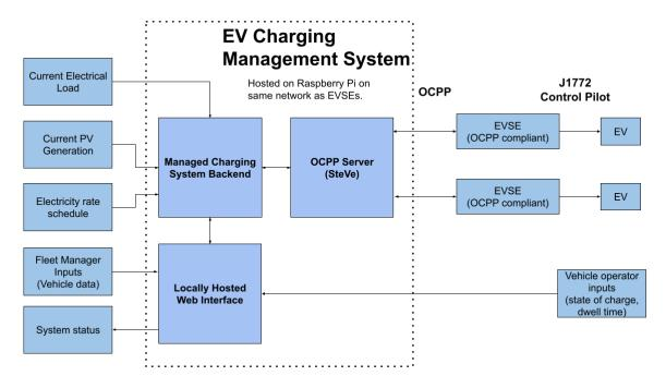
Figure 2.1. Software System Architecture
