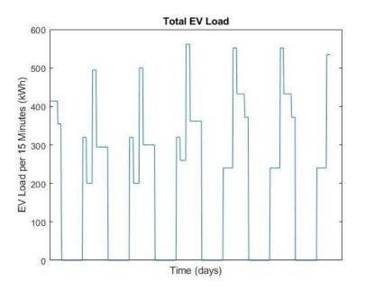
Figure 2.5. Power Schedule for the UW Transportation Electrified Fleet
