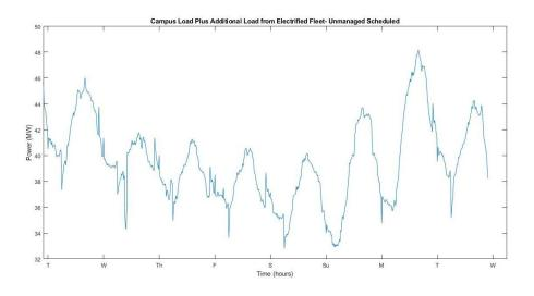
Figure 5.6. Total Load for Unmanaged Scheduled Charging
