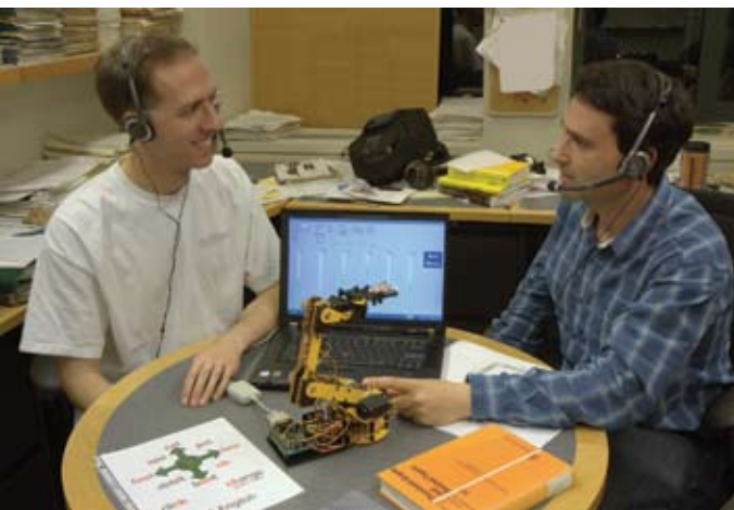
Graduate student Jon Malkin & Associate Professor Jeff Bilmes use the Vocal Joystick to control movement of a robotic arm. The computer screen shows how the software analyzes vocalizations to create instructions for the arm’s movement.
