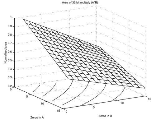
Fig. 11. Multiplier area vs. number of zeros substituted
