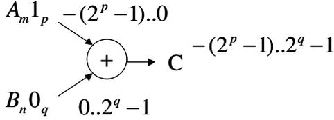
Fig. 3. Normalized error model of an adder
