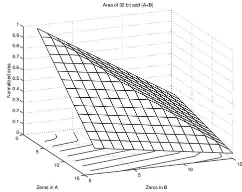
Fig. 6. Adder area vs. number of zeros substituted
