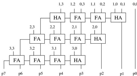
Fig. 10. Multiplication hardware requirements
