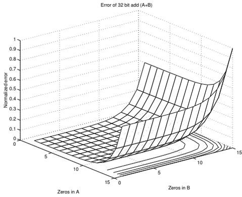
Fig. 8. Adder error vs. number of zeros substituted
