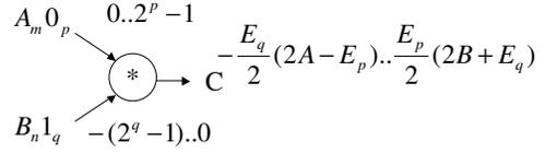
Fig. 4. Normalized error model of a multiplier
