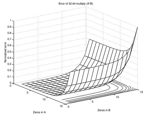
Fig. 12. Multiplier error vs. number of zeros substituted
