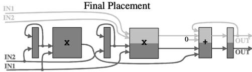
Fig. 5. Final placement of the architecture created from the initial placement in Fig. 4. The signal cross-section has been greatly reduced during the placement process.
