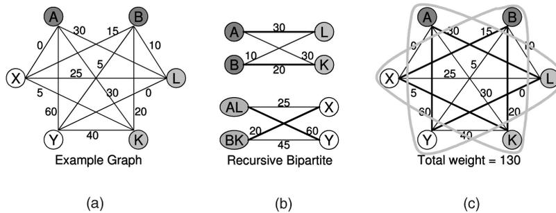
Fig. 7. Recursive bipartite matching for these three netlists results in a suboptimal solution. Nodes are signals (shades indicate netlist), circled groups are wires, and the cost is the sum of the edge weights in the groups. (a) Graph, (b) recursion steps, and (c) solution.
