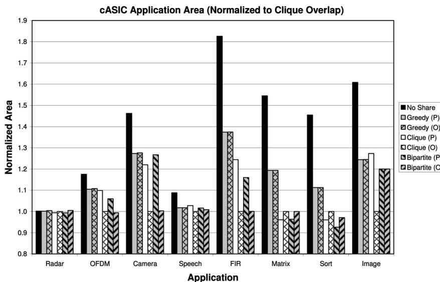
Fig. 9. Comparative area results of the different cASIC routing generation algorithms, normalized to the Clique Overlap result for each application. The Bipartite results given are the average across orderings.
