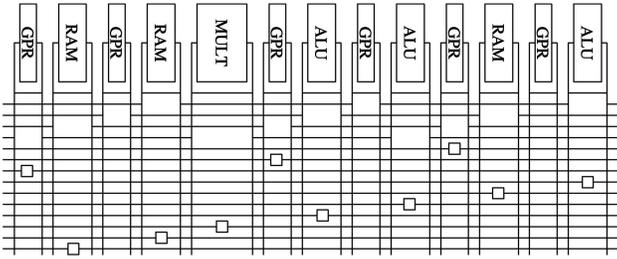
Fig. 1. A single cell of RaPiD [17], [19]. A full architecture is composed of multiple cells laid end-to-end.
