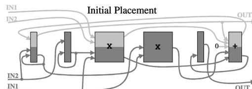
Fig. 4. An initial physical placement and binding for an architecture for the Fig. 3 netlists. Shading shows component use by netlist, but only one can be active at a time.
