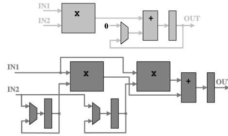
Fig. 3. Two example netlists for architecture generation. The light netlist performs a multiply-accumulate (MAC), while the dark netlist is a 2-tap FIR filter. These two netlists are used in the example placement process given in the next few figures.
