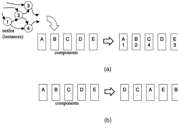
Fig. 2. Binding versus physical moves. (a) *Binding* assigns instances of a netlist to physical components. (b) *Physical moves* reposition the physical components themselves.
