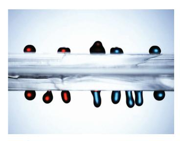
Drops of red and blue liquid move along the upper and lower surface of the vibrating UW platform at speeds up to 1 inch per second. This combined image shows drops as they move toward the center and merge. Copyright 2012 Wiley.
