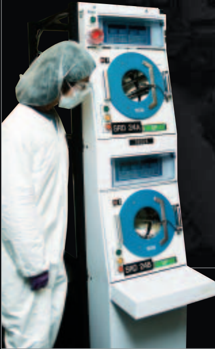
GRADUATE STUDENT SHIHO IWANAGA CLEANS SILICON WAFERS IN A SPIN-RINSE DRYER IN THE EE MICROFABRICATION LABORATORY.
