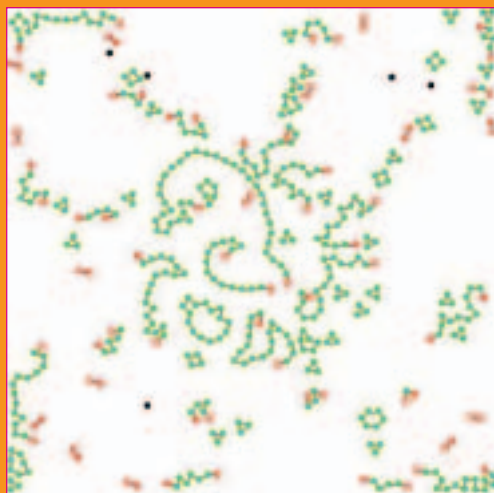
A SIMULATION OF "PROGRAMMABLE PARTS" ASSEMBLED INTO STRANDS AND RINGS. THE PARTS FLOAT IN A (SIMULATED) FLUID MEDIUM. UPON RANDOM COLLISIONS, TWO PARTS MAY CHOOSE TO ATTACH TO EACH OTHER OR NOT, BASED ON THEIR PROGRAMMING.
