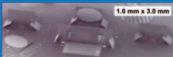
SEM OF A MEMS POLARIZATION CONTROLLER THAT CAN ACHIEVE FAST AND STABLE CONTROL WITHIN THE ACCURACY OF ONE WAVELENGTH.
