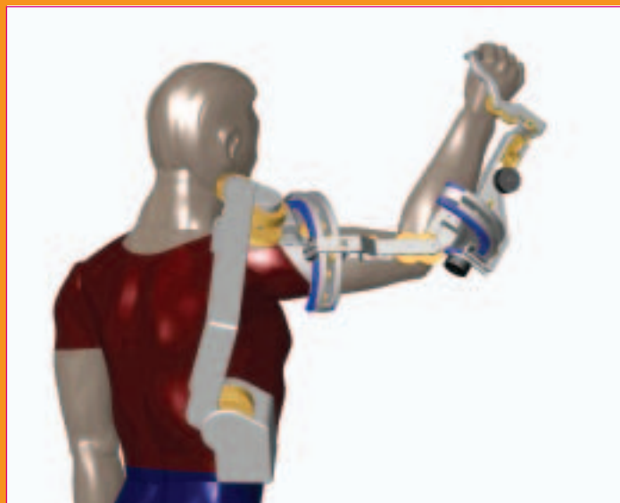
EXPOSED VIEW OF UPPER LIMB POWERED EXOSKELETON WITH 7 DEGREES OF FREEDOM.
