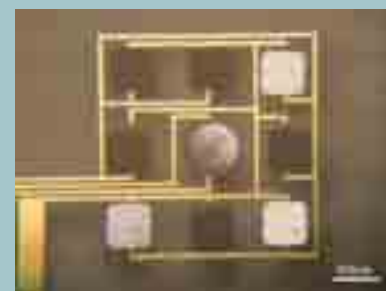
Self-assembled detection unit consisting of a circular LED excitation source surrounded by square silicon photosensors.
