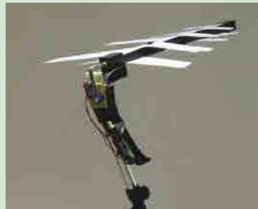
A prototype test rig was constructed to demonstrate harvesting from a cellular base transceiver station. The antenna used for these tests was a typical broadband UHF digital television antenna with 6 dBi gain.
