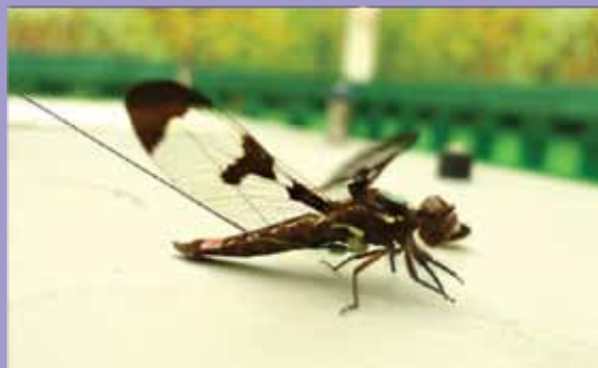
A dragonfly with the wireless recording system attached to its thorax.
