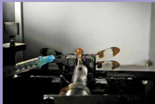
Implanting a microelectrode array into the dragonfly's nerve cord.
