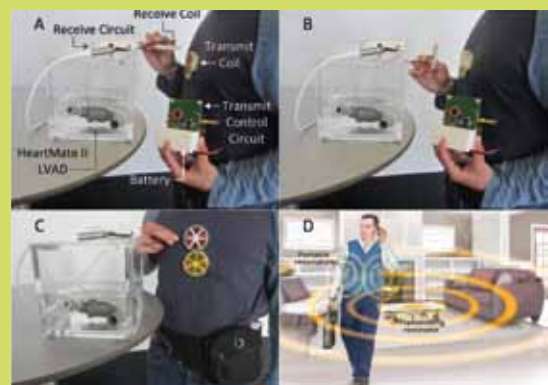
Demonstration of the battery-powered portable transmitter system used to wirelessly power a commercially available axial LVAD using two equivalently sized transmit and receive coils in a (A) perpendicular configuration, (B) parallel configuration, (C) and side-by-side configuration. (D) A rendering of the FREE-D system vision for a wireless, in-home VAD system.
