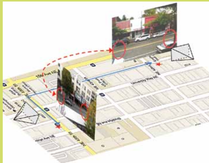
An example of connected zones identified. Red stars denote the camera locations. Red ellipses are the entry/exit zones. The connected zones linked by the red line can be identified based on the principal orientations and the direction of the route (shown as the blue line).
