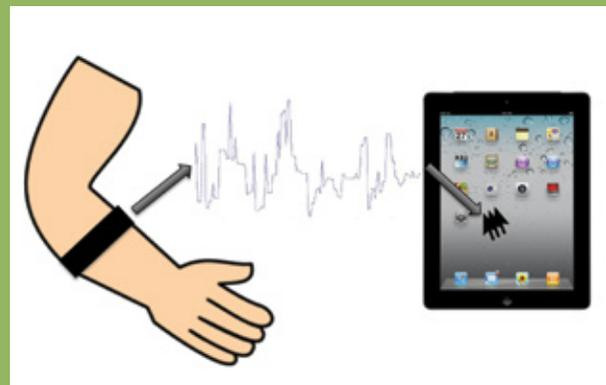
Using a band of electrodes (pictured here on an arm), electromyography (EMG) signals are translated into a virtual cursor that replaces fingertip gestures. The EMG signals can also be measured from other muscle groups, such as the neck.
