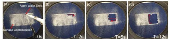
Water droplet cleaning surface contaminants with zig-zag layout of ARC surface
