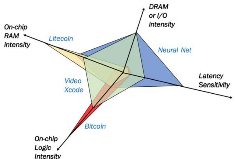
Taylor's prototypical ASIC Cloud Architecture explores applications with varying accelerator properties.
