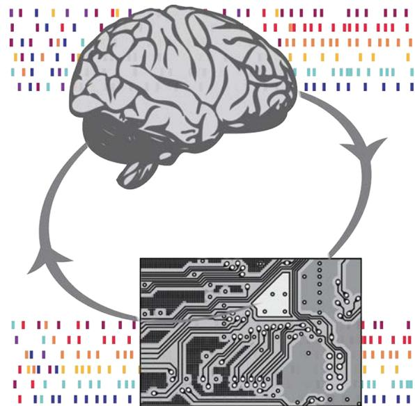
**BMIs record neural activity into a control signal for an actuator via the "decoder," or algorithm. Feedback of the actuator movement creates a closed-loop system. BMI performance is shaped by both the decoder and the brain.**
