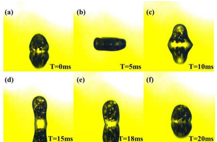
2.9  $\mu$ L water droplet carrying 2mg sand particles while moving along ARC surface
