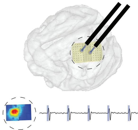
**Schematic of the novel optogenetic interface for NHPs that enables stable, large-scale stimulation and recording across cortical areas (top). Examples of spatial (bottom left) and temporal (bottom right). The blue rectangles represent the duration of light stimulation, light-evoked neural responses. This interface offers a powerful tool for studying stimulation-based neurorehabilitation.**
