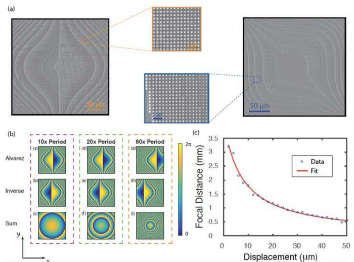
**Dielectric metasurface freeform optics:** (a) SEM of the fabricated cubic phase-plates, which together can form a composite Alvarez lens. (b) By laterally displacing these two cubic phase-plates we can realize lens-like (quadratic) phase profile with varying curvature, and hence different focal lengths. (c) Experimentally measured focal length as a function of the lateral displacement, showing the nonlinear change in the focal length.
